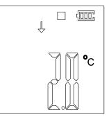
⑧Temperature: Below Lower Limit (Stop recording status)
