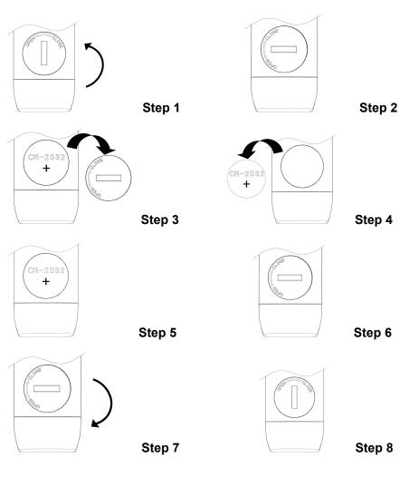
Step1: Turn the battery cover anticlockwise to open it. Step2: The battery cover position is as shown, indicating that it has been rotated to the accordant position. Step3: Take off the battery cover.
