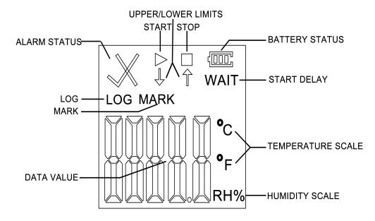
During normal recording process, shortly press "▶" to switch to different display interface. The interfaces shown in sequence are respectively:
